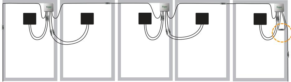
The shortest pair of input leads should be connected to the first panel of each pair.
